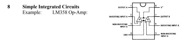
Integrated circuits typically contain a large number of circuits embedded on a single chip. They are each designed for a specific function, and are generally mass-produced by the thousands or millions. They come in different packages – this class uses chips in the dual in-line pin (DIP) package that fits into a plastic solderless breadboard.
